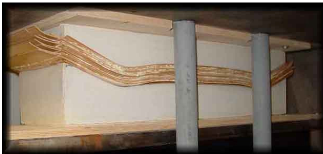
Figure 2.2.2: Maple veneers in a hydraulic press
